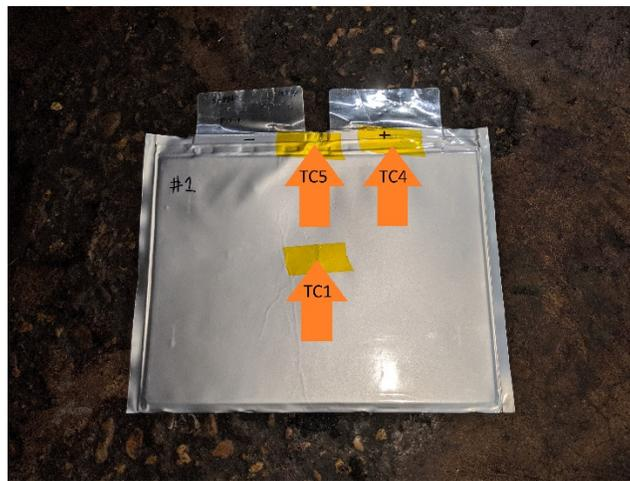
Figure 4 – Initiating thermocouple locations
