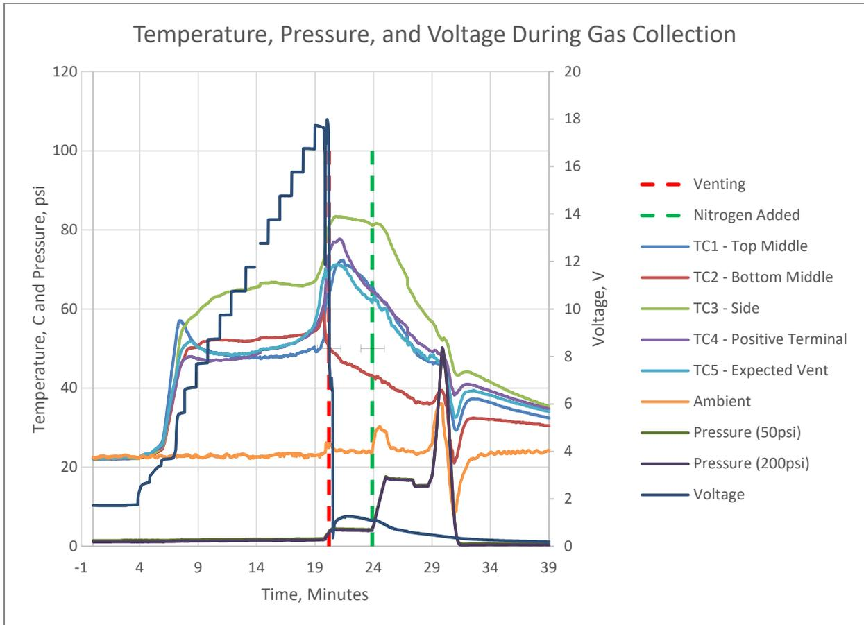
Figure 25 – Surface temperatures measured on cell
