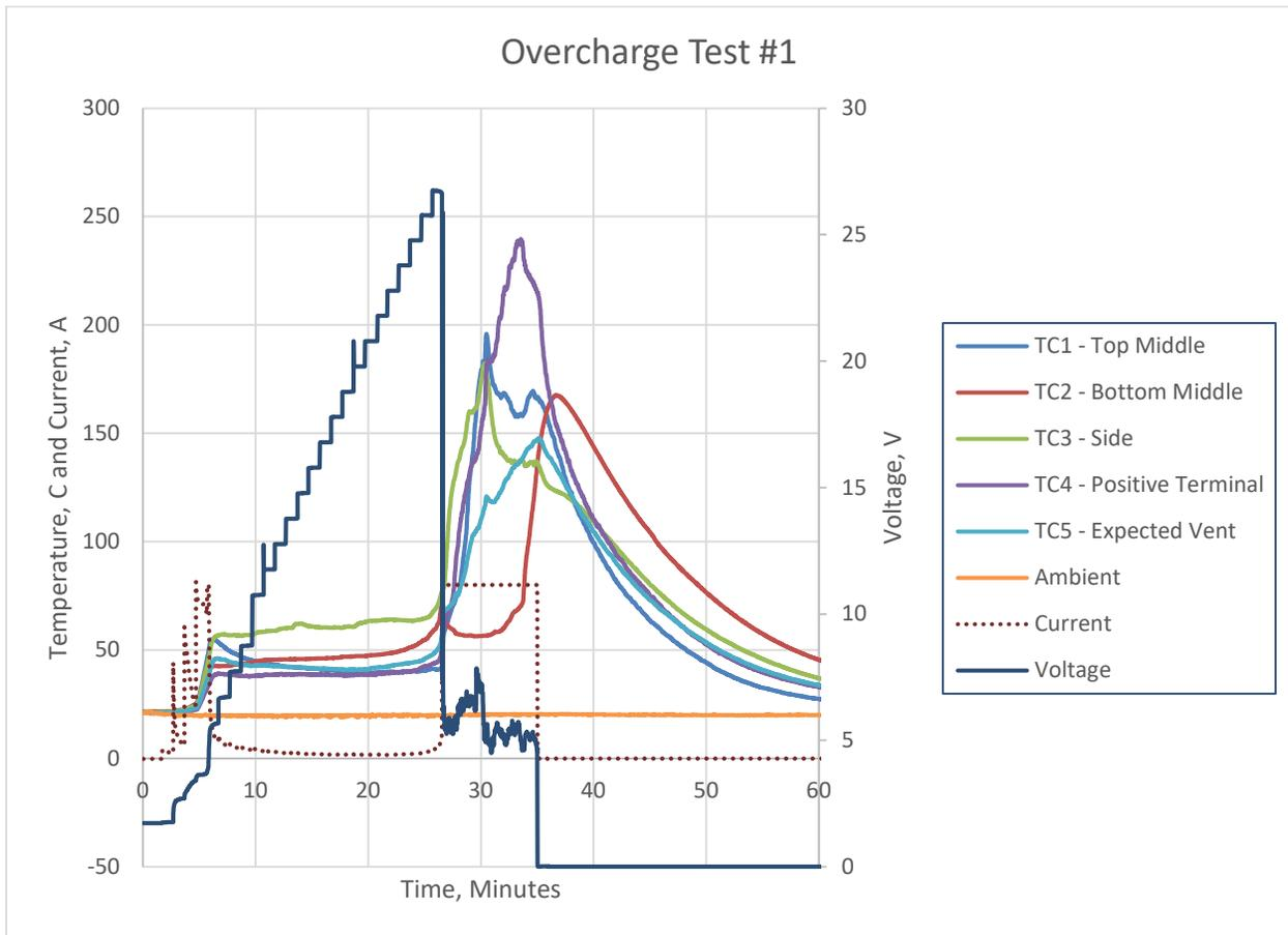
Figure 13 – Surface temperatures measured on cell
