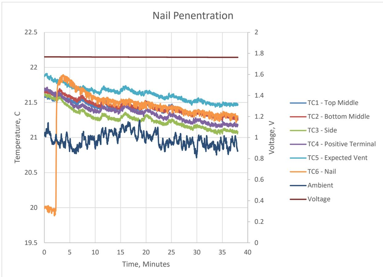
Figure 16 – Surface temperatures measured on cell
