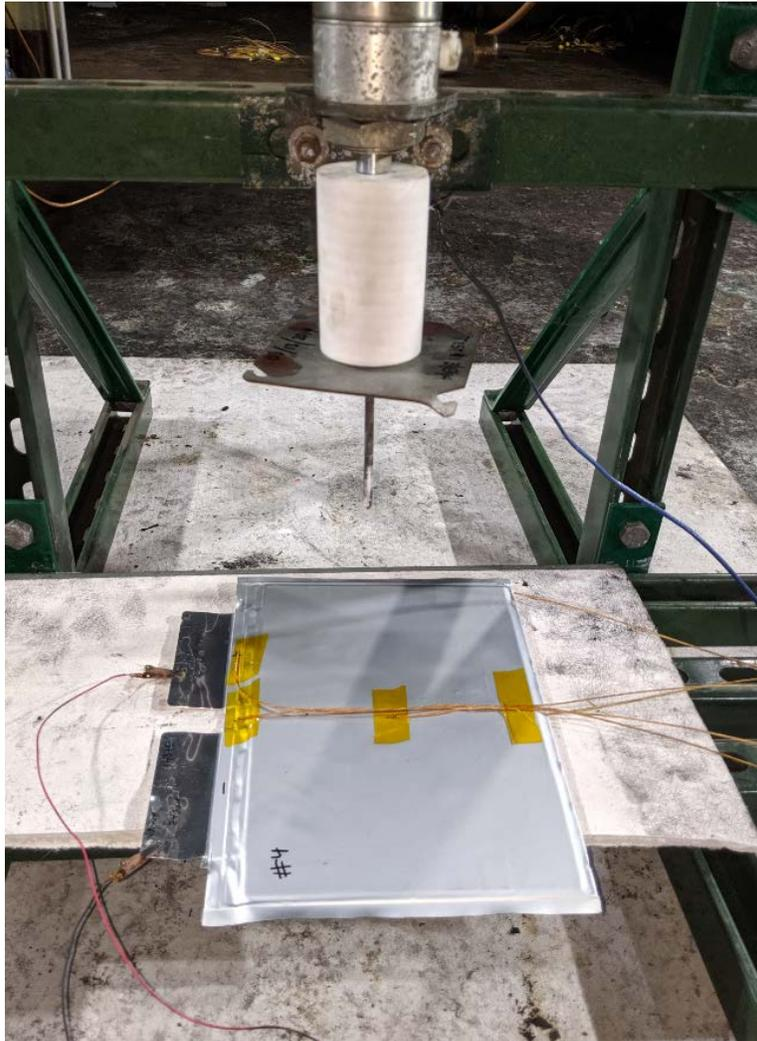
Figure 17 – Nail Penetration Setup
