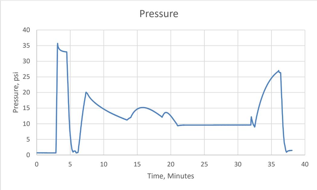
Figure 24 – Pressure inside the cell gas composition test chamber before overcharging
