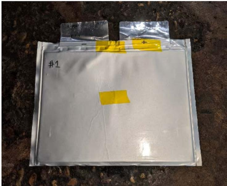
Figure 7 – Photograph of cell after test
