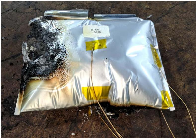
Figure 15 – Photograph of cell bottom after test
