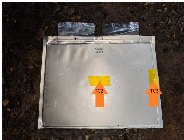
Figure 5 – Additional view of thermocouple locations
