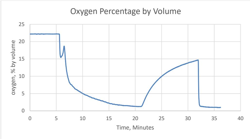
Figure 23 – Oxygen concentration during purge of cell gas composition test chamber prior to start of test
