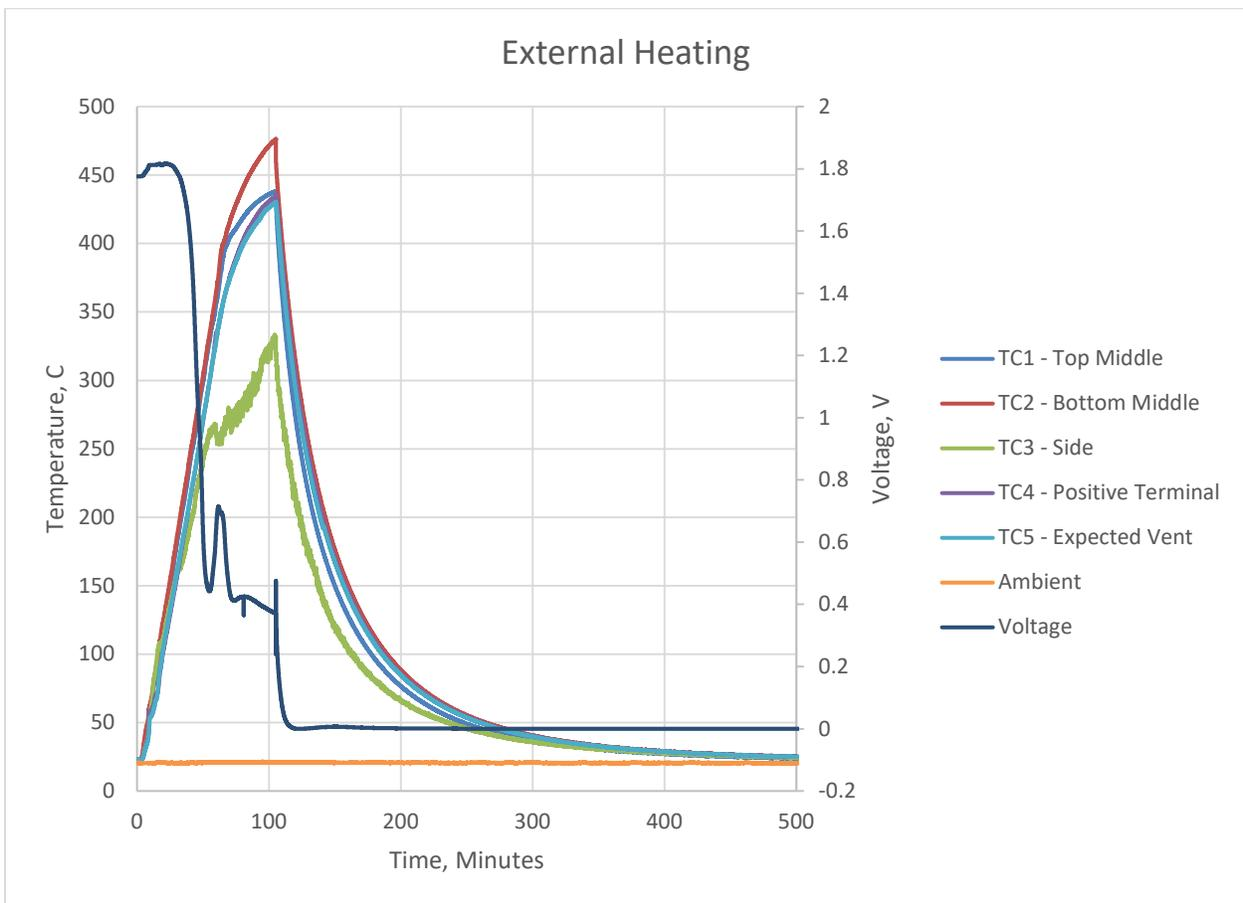
Figure 9 – Surface temperatures and electrical parameters measured on cell
