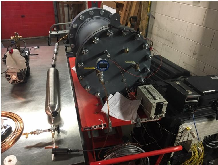
Figure 22 – Cell gas composition test chamber
