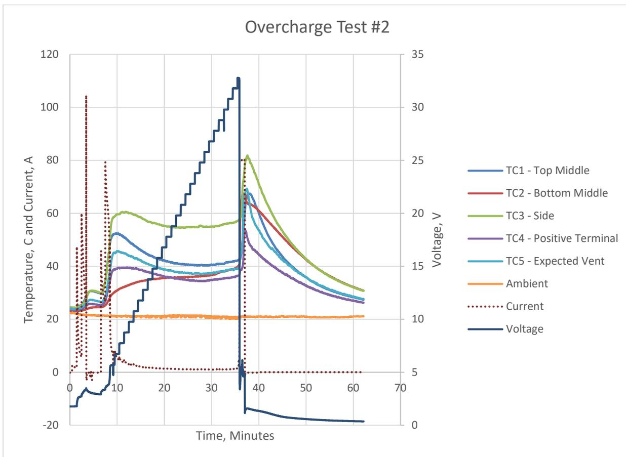
Figure 19 – Surface temperatures measured on cell
