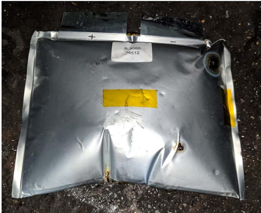
Figure 21 – Photograph of cell bottom after test
